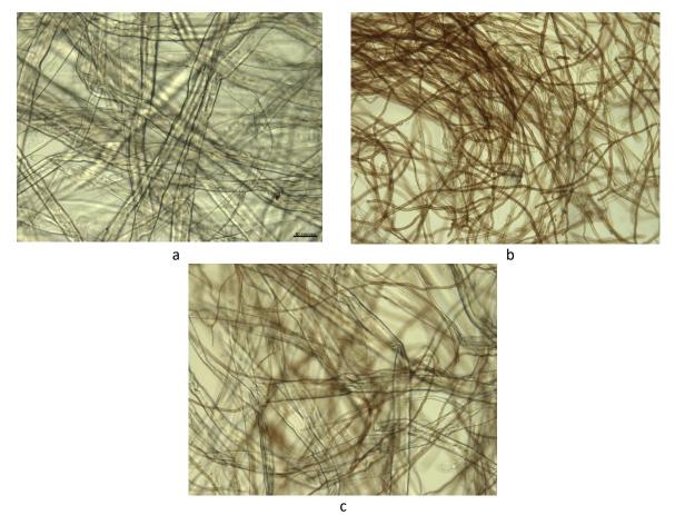
Figure 5. KF fibres 30  $\mu$ m in diameter (a), fungal fibres (hyphae) 3-6  $\mu$ m in diameter (b) and composite material KF FF 50/50 (c); LM 200x
