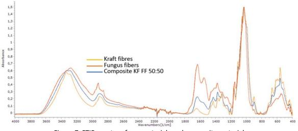
Figure 7. FTIR spectra of raw materials and composite material.
