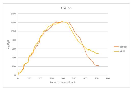
Figure 8. Biochemical oxygen demand during the incubation of KF FF 50/50 in the substrate
