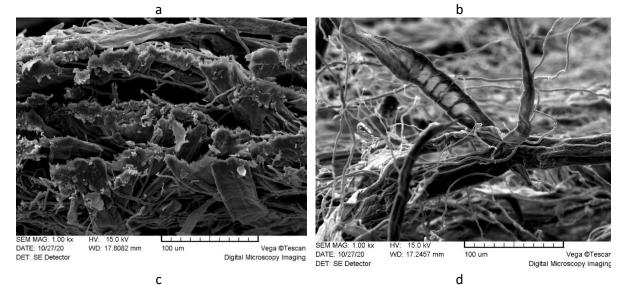
Figure 6. SEM microscopy of fungal hyphae and cellulosic fibre composite material membrane: a,b surface structure; c – cross section, cut; cross section, torn.
